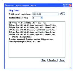
Figure 8-43: The Ping Test
